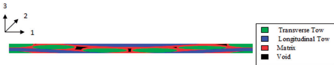
Figure 3. 2D Unit cell of 5 harness satin composite.
