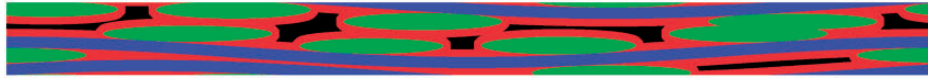
Figure 11. Representative volume element with tow offset equal to 4.5. Note the difference in void sizes and shapes.
